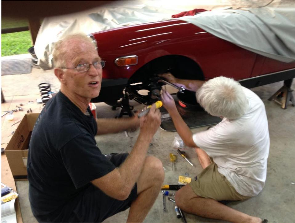
Cleaning the stub axle parts was a major pain and very time consuming but worth it and in the end the stub axles, kingpins and top trunnions all proved to be in good shape.
