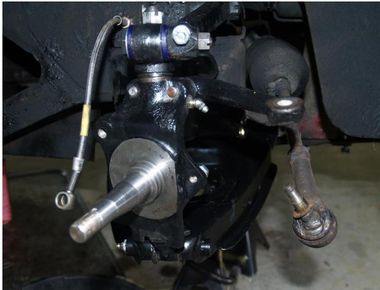
Next the old track rod ends and gaiters were removed. The outer ball joints cleaned and... greased and new gaiters fitted.
