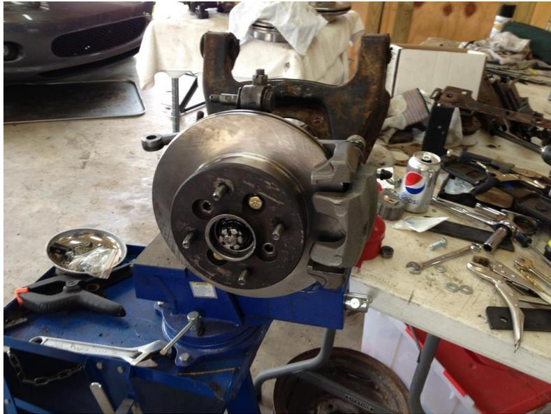
Charlie designed a simple caliper adapter plate for the holes for the Midget spindle and located the holes for the caliper using a piece of stiff fiberboard for a template. After adding a couple spacers for the bolts, everything fit together as planned.
