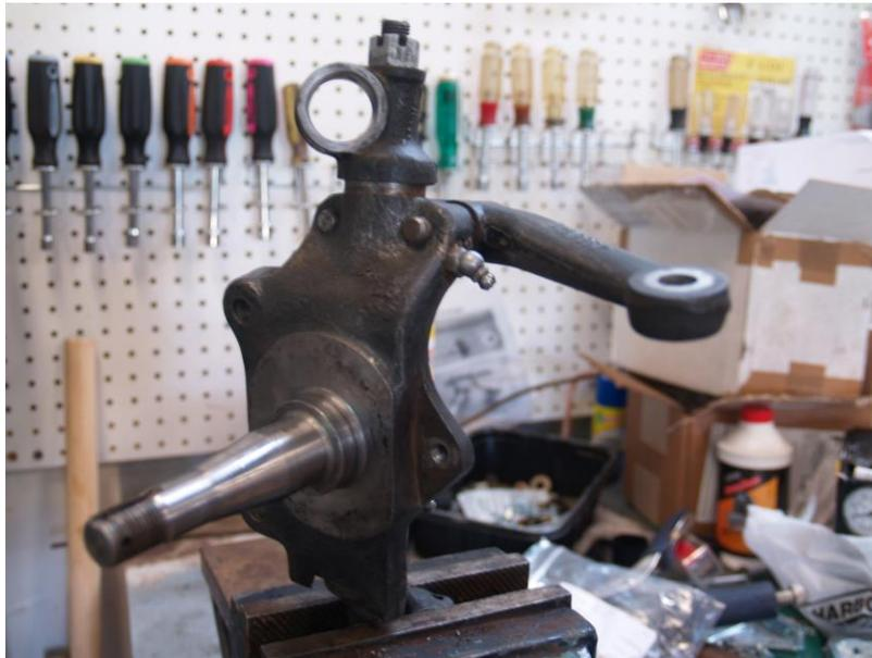
I used the original shims but had to replace the oilite thrust washers with new ones to remove end play. The kingpins felt smooth with no wobble so the axles did not require rebushing thank goodness!
