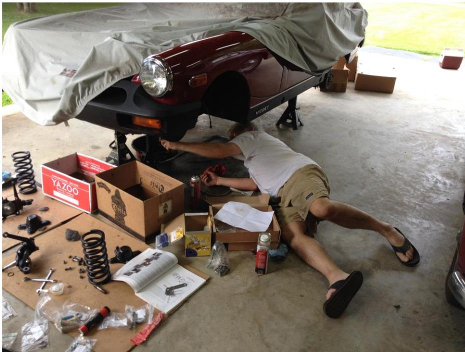
The damaged wishbones went in the trash bin and were replaced with new ones from British Motor Heritage. I decided to use all new fasteners and fittings but did keep the original dust excluders and springs. After cleaning, all the parts were either polished or primed and given several coats of chassis paint including the springs, spring seats and rotor back plates.
