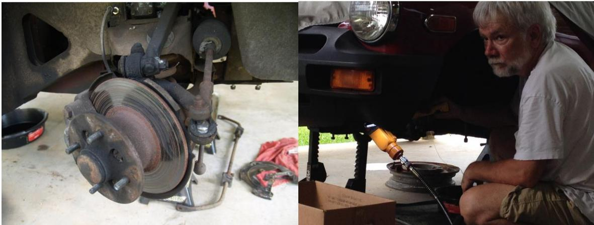
The rubber bushes were all in bad shape, some nearly worn through. The rotors, being original, were slightly less than minimum factory thickness - time to replace them too. Track rod ends were in bad shape and the gaiters were split to boot...pun intended. After releasing the top trunnions and track rod ends from the steering arms you can see the accumulated old grease and road grime on the stub axle assembly. A thorough scrubbing was in order.
