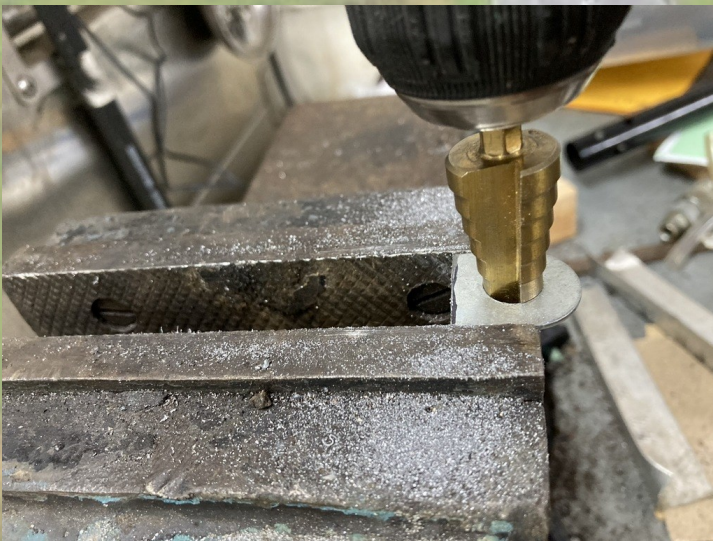
Drilling the tab to size
