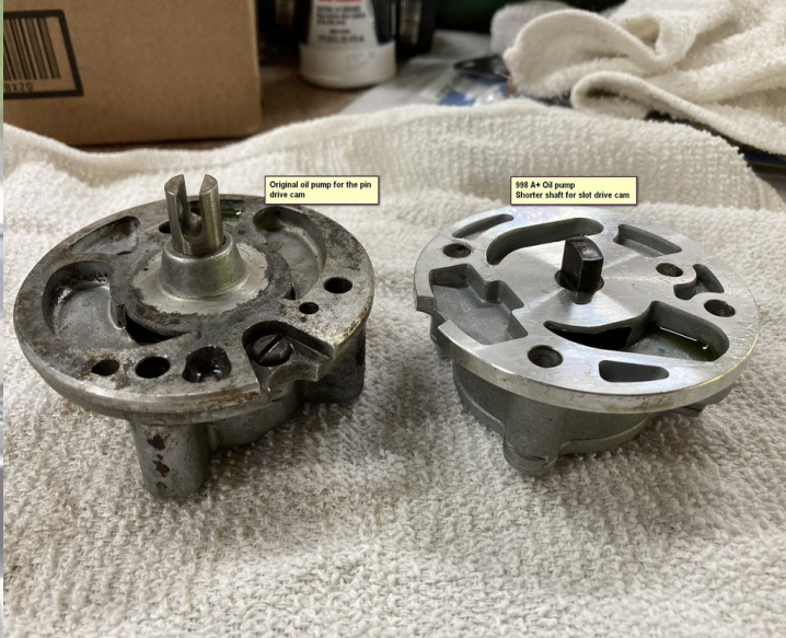
Oil pump drive ends
