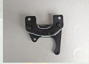
Once the new brackets were made it was simple to get the 240SX calipers mounted to the GT. In addition to more rear bias the 240SX did not require reshaping the park lever and I much prefer the position of the park lever for clearance reasons.
