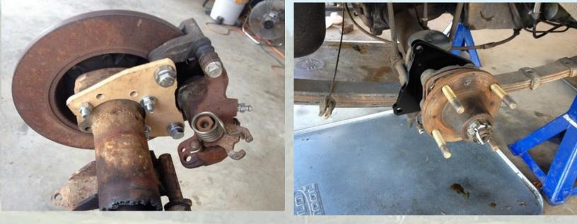
Once all of that was established I had a CAD drawing commissioned. With a CAD drawing in hand my next stop was to the machine shop with laser cutting equipment. 2 weeks later I had two brackets ready for fitting to the spare axle housing.
