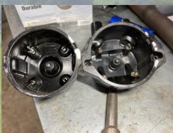
Arching to side of terminal of old cap
