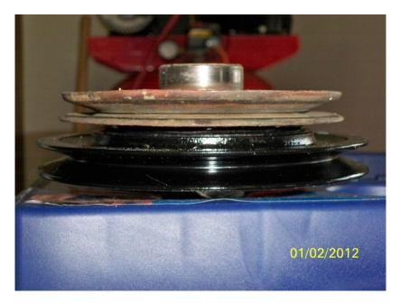
Before the head went back on I took the time to confirm that TDC on the crank pulley is in the proper place. It's an easy task if you have a dial indicator. The same job can be accomplished with a flat piece of metal and a bolt.
