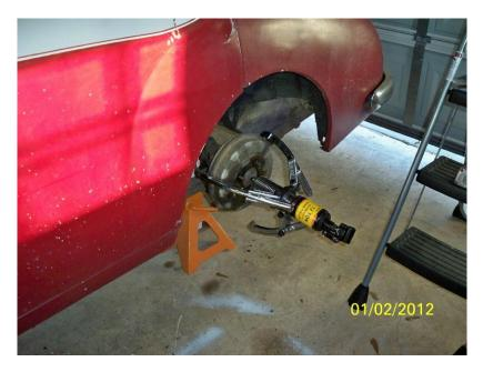
Once the drums were off I found that 1 return spring had come off. Too bad the shoes were ruined by the leaky brake fluid. The previous owner had installed new shoes without properly servicing the wheel cylinders. That's it for now. The Chick Magnette will live again.
