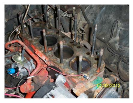
The head was in similar condition. The mating surfaces were cleaned and the head was ready to reinstall.
