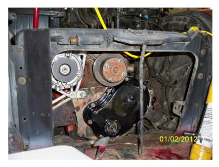
Another benefit in changing from the original Magnette pulley is that the MGB pulley takes a much wider  $\frac{1}{2}$ " belt. The original 5/16" belt may have been good for driving the old 15 amp alternator but that simply would not do with the 65 amp alternator conversion.
