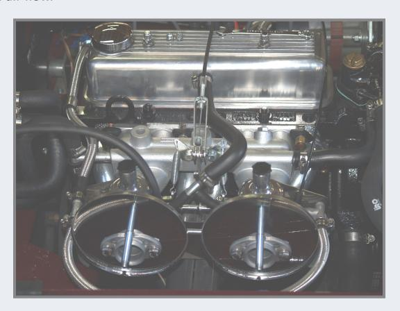
Finally the filters and carb to carb fuel line was installed. I decided to use stainless line for this.
