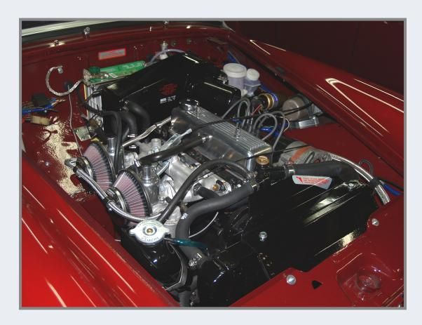
With the charcoal canister removed I decided this was a good location for a Tudor washer bottle. Originally a plastic bladder had been installed and mounted under the opposite fender.
