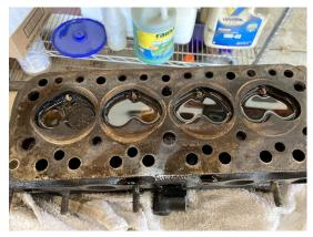
With the head off the valve seal could be tested. The head was turned upside down and the chambers were filled with solvent. It took a while for it to become obvious that there is a leaky valve when the solvent drained from the #4 combustion chamber. With solvent draining from the exhaust port, the #4 exhaust valve seal must be compromised.
