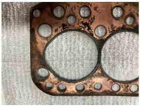
A close inspection of the head gasket revealed the source of the coolant leak. The source of the leak was at the rear of the head gasket and the coolant had wicked around to the side. The gasket also revealed evidence combustion seepage around all of the cylinders. Clearly, disaster has been averted.
