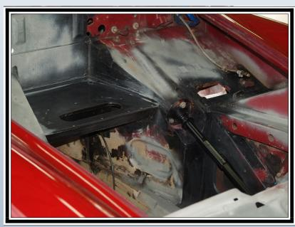
The hole in the bulkhead has been patched and filled. Any suspicious areas were treated with POR 15 corrosion inhibitor. Bare metal was sprayed with self etching primer. The steering rack and column were given several coats of chassis paint and every surface was lightly sanded and wiped repeatedly with paint prep.
