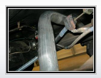
I ended up fixing the routing by cutting and re-bending the pipes myself. So much for using the pros for an unusual application.
