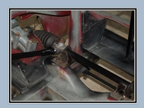
I took advantage of Greg Matheny's welding workshop to replace the footing on the rear heater box panel as the original had suffered badly from battery acid corrosion.
