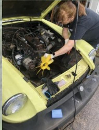
Margie Hollingsworth has been working on her 76 MGB. She replaced the radiator and rebuilt the ZS carb. She also replaced all of the associated hoses. All she lacks is replacing the steering rack gaiters and adjust the toe in to be road worthy for a spirited drive with EMC. Good job Margie
