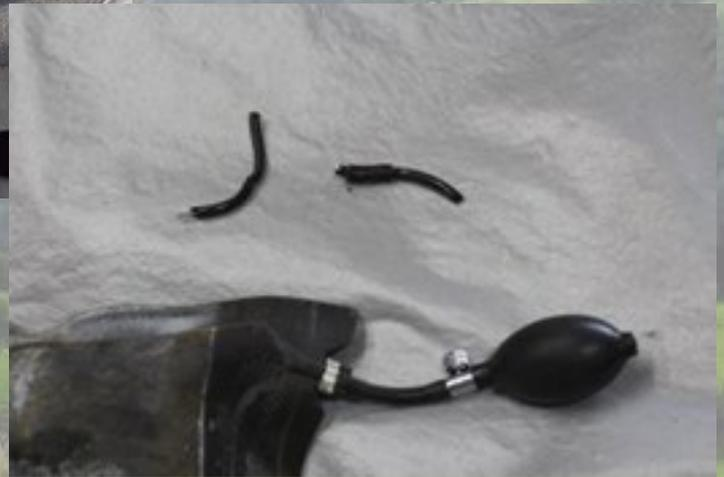
Since originally only the driver's side had the support system, I decided to see if I could retro fit the passenger side. None of the state-side Lotus Parts had any in stock and getting from England seemed particularly expensive I came up with the idea to use a Lock Picking bladder to use on the passenger side and use the parts from another to repair the driver's side. I ordered two from a supplier in China (Holy Churchill, a Chinese part in a Federal English car).
