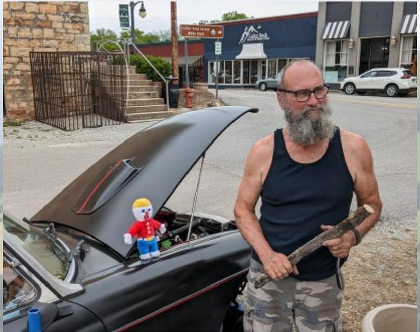
was able to diagnose the problem as a broken starter bolt, allowing the starter to swing away from the flywheel, and solved it with a piece of tree branch strategically placed to wedge the starter! On to Jojo's for catfish, then off to Mountain Home for the night.
