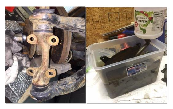
So I tried another successful YouTube inspired method of vinegar rust removal. Using 2 gallons of white vinegar (\$2.48 each at Walmart) I poured it into a plastic bin with enough to cover the rusty parts. Any part left exposed seemed to rust more so some parts got flipped over several times.
