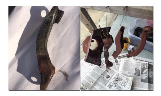
After 24 hours in the vinegar bath I removed them and scrubbed them with with steel wool and water. It worked! I used a Lowe's product of Rust-oleum for metal priming and protective black enamel—about \$25 for each gallon. The parts look great and are ready for reassembly with some new bushings.
