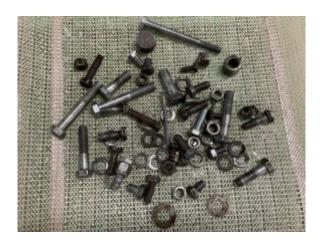
For the last 2 batches I added straight Super Clean and then straight EvapoRust. The label on the Super Clean claims it's the best there is so way not give it a try. For this test I ran the tumbler for 1 hour. I found that the Super Clean is tough to rinse off and frankly did not clean much better than water/soap.
