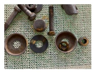
In conclusion, the tumbler does a pretty good job using soap and water. A 2 hour tumble seems to be about right with a splash of WD40 on the rinsed parts. Now on to the rest of the parts in the bucket for a fun day(s) of tumbling.
