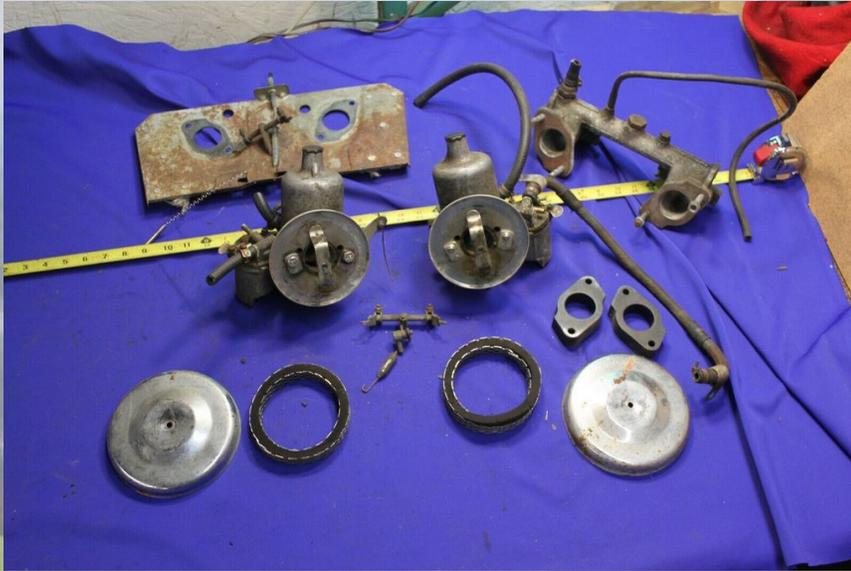
The original carbs were AUD135. The reason for the change is the AUD135 carbs do not have a PCV port. The replacement carbs are AUD465. The AUD465 does have a provision for a PCV without using the Smiths PCV valve that is used with the AUD135 carbs.
