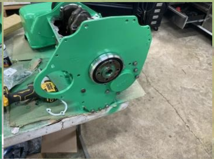
Seal kit installed
