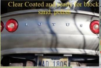
The finished repair came out great. I only have to block sand the clear coat and polish. After a little wax the repair will be undetectable to most eyes.
