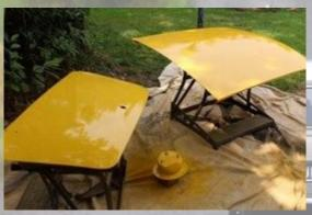
Followed up with three medium coats that I felt gave good coverage. I let it sit for about 2 hours outside and moved the pieces inside the garage at they felt touch dry. Upon closer examination, I only found one run and a couple of bugs that sacrificed their lives to test the tackiness of the paint. Since the paint was a little thick I experienced a slight orange peel. After completely drying, I should be able to block sand and correct any problems so far.
