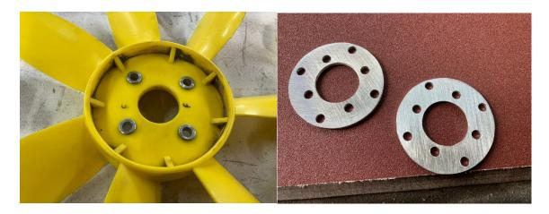
Since the new orange fan is nylon, it is made of a compressible material. I am not comfortable with just a bolt head holding the fan in place without some reinforcement. My solution was to make a clamping ring to spread out the load and the use of blue LocTite to keep the bolts from backing out unexpectedly.
