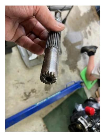
Not to be defeated Brother Clay and Charlie modified a spare input shaft that was on hand to allow the reaming of the pilot bushing in place. After 30 minutes of work, we were successful in cleaning up the pilot bushing and on the first attempt the transmission slid into place. The engine/gearbox assembly was re-installed.
