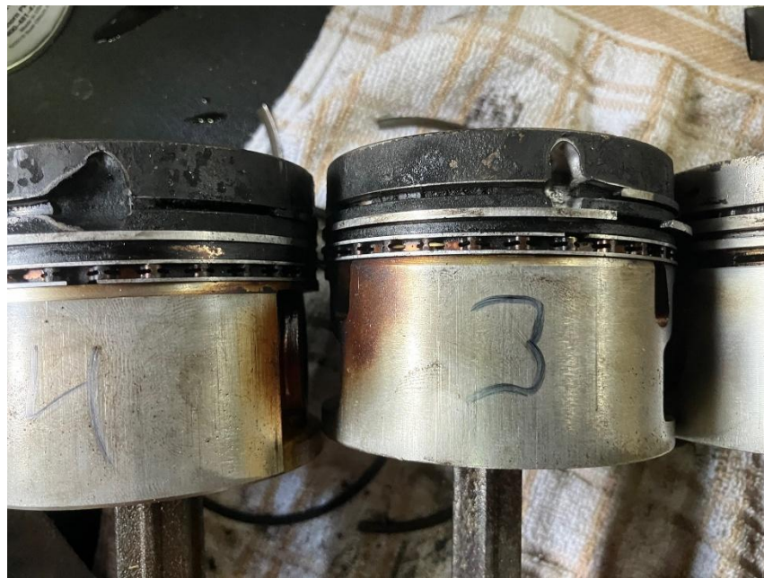
Pistons 3 and 4 with damage
